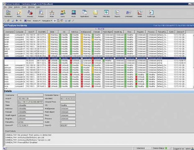
ConSentry InSight Command Center provides a single focal point for administering and monitoring EPV policies and events that may be operating on multiple ConSentry LANShield Switches and Controllers, increasing IT's efficiency and lowering its OPEX. IT can use InSight to create and distribute global policies defining PC health criteria, quarantine policies, remediation steps, and warning messages.
